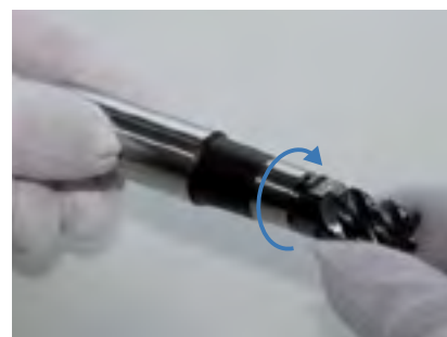
3. Screw the replaceable milling head into the replaceable head holder, turning it tightly by hand. Then, screw the replaceable head holder, along with the tool, into the machine holder.
