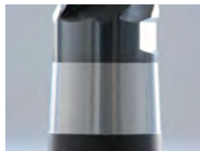
3. Screw the replaceable milling head into the replaceable head holder, turning it tightly by hand. Then, screw the replaceable head holder, along with the tool, into the machine holder.
